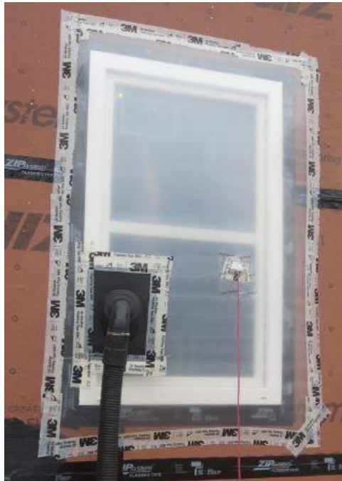
A simple mock-up could be the first window installed on the project.
