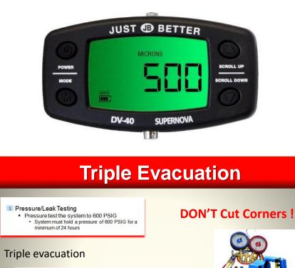
Evacuate the system to 4,000 microns from both service valves (where available). System manifold gauges must not be used to measure vacuum. A micron gauge must be used at all times
