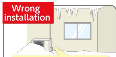
Unit may become buried in snow due to heavy snowfall, snow sliding off the roof or snowdrift. Line Set Installation
