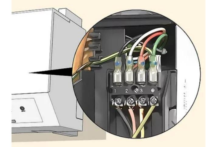
Install 3-pole disconnect switch, in order to deenergize the indoor unit for service or repair.
