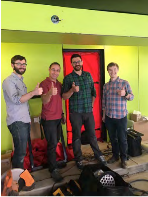
FINAL BLOWER DOOR TEST Sept 29, 2017 .53 ACH50
