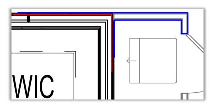
Red = sealed air barrier layer. Blue = finished sheetrock that does not maintain an air barrier.
