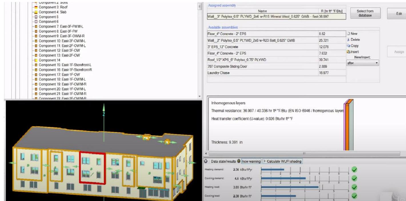
The screenshot displays the WUFI Passive software interface. On the left, a 3D model of a building is shown with various components highlighted in yellow and red. A central vertical axis indicates the orientation. To the right, a list of components is visible, including:
